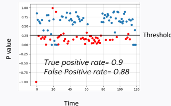
Fig1: Blue dots are benign CAN packets and red dots represent anomalies.
