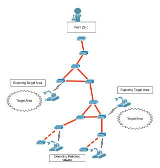
Figure 4: Concurrent search and expansion with multiple robots.
