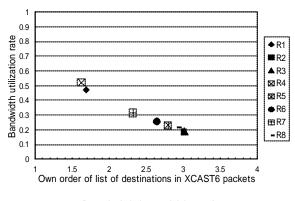
Fig 11 Bandwidth utilization rate at the order of the list of destinations
