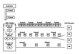
adopted the TCP-friendly Rate Control protocol (TFRC) [7] approach. TFRC is an equation base congestion control method for unicast applications which provides smooth rate control while maintaining fairness with other TCP traffic competing with the flow.
