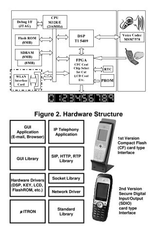
Figure 3. Software Structure and Appearance
