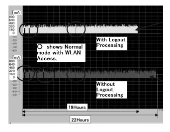
Figure 13. Battery consumption
