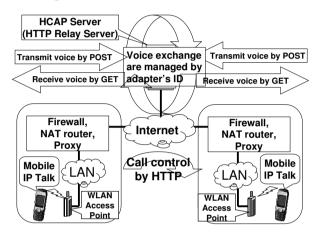
Figure 5. IP Telephony Structure with HCAP Server(HTTP Relay Server)
