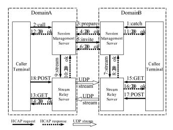
Figure 6. Basic Example of HCAP Call Control
