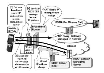
Figure 9. HCAP Solution for SIP Communication with Dynamic Global IP Address
