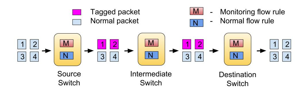
Figure 1: Packet Tagging Mechanism
