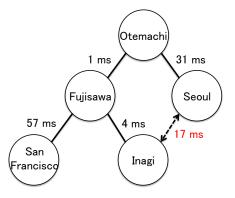
Fig. 1: Current Layer 2 over IP based Layer 2 network extension technologies limit the topology to a tree
