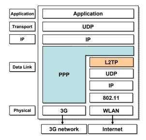
Fig.5: Protocol Stack of PPP Extension
