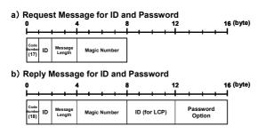
Fig.8: ID / Password Request and Reply Message
