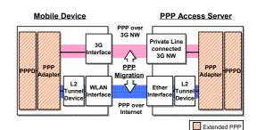
Fig.2: System Components
